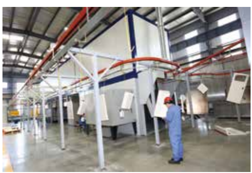
Automatic powder coating lines ▼
